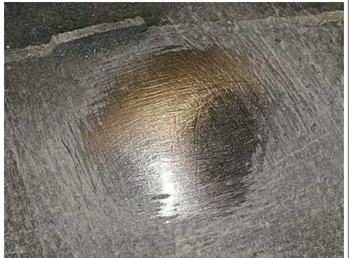
Final inspection – GFK [NO cracks]
