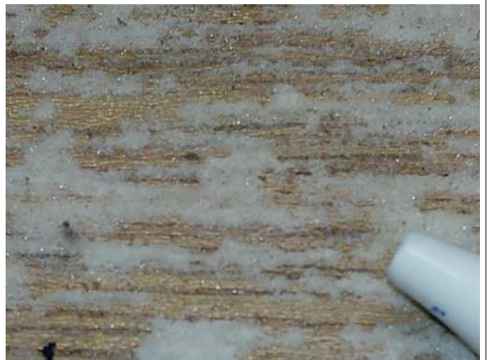
Final inspection – GFK [with cracks]
