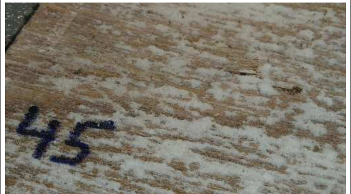
Final inspection – GFK [with cracks]
