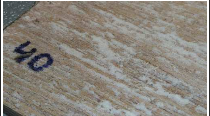
Final inspection – GFK [with cracks]
